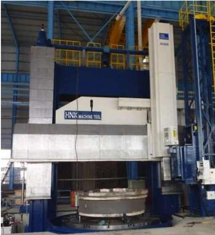
Component : Casting & Machined Runner Band Customer : Alstom Hydro Material : CA6NM
